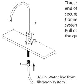
Thread the quick connect adaptor (F) onto the end of the faucet assembly (A) stud, and tighten securely using a wrench.
