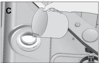
4. Fill the salt reservoir with salt by using the salt funnel (D). To speed up dissolution rate of salt in water, stir it with a spoon.
