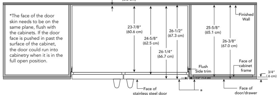
\*The face of the door skin needs to be on the same plane, flush with the cabinets. If the door face is pushed in past the surface of the cabinet, the door could run into cabinetry when it is in the full open position.
