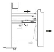
2. Remove the tray (B) by lifting it up, and out, as shown below.
