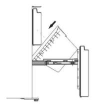
2. Put the tray on top of the drawer, and push it inward to enusre the tray's rollers are set on the freezer liner.
