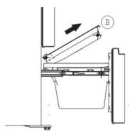
3. Remove the freezer drawer by lifting it up and out of the unit.
