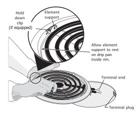
Figure 14: Removing coil and drip bowl
