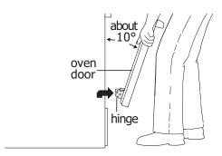
Figure 19: Holding door for removal
