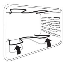
Figure 15: Lift bake element
