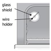
Figure 21: Oven light protected by glass shield
