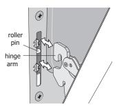
Figure 20: Replacement and location of hinge arm and roller pin
