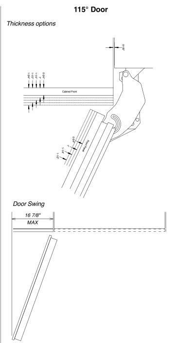
NOTE: Additional space needed depending on the thickness of front panels and handle used. Freezer units cannot be stop pinned at 90°
