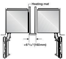
In this case, you will only need the heating mat from the "Merging Kit" to avoid condensation and prevent damages
