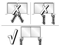
If the appliances are installed directly next to each other (without a partition), they need to be attached together. A heating mat must also be installed. This will help avoid condensation and prevent damages.
