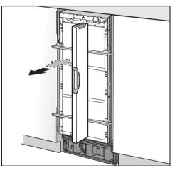
Align the appliance again using a level.
