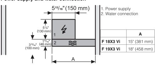
Install a pressure limiting device and water hammer arrester for inlet water pressures exceeding 80 psi.(Refer to Uniform Plumbing Code, Sections 608.2 and 609.10) Never install or operate where inlet water pressure may exceed 120 psi.
