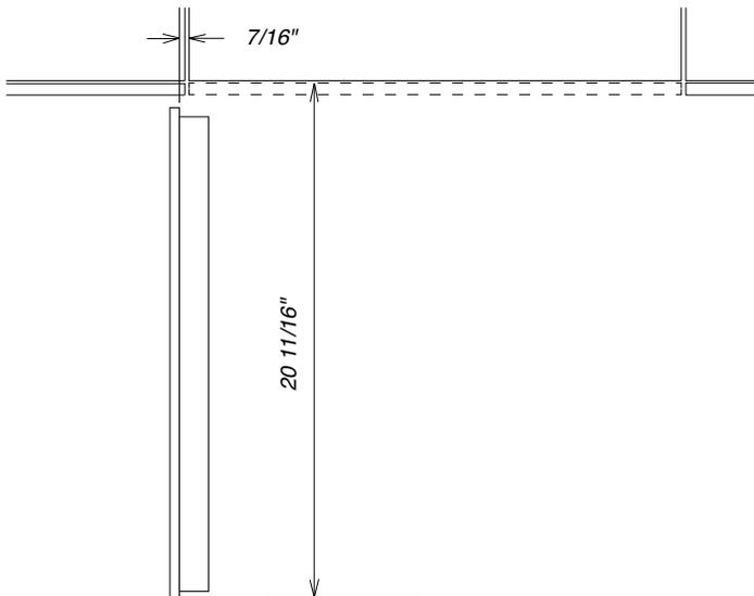
**NOTE:** Additional space needed depending on the thickness of front panels and handle used.
