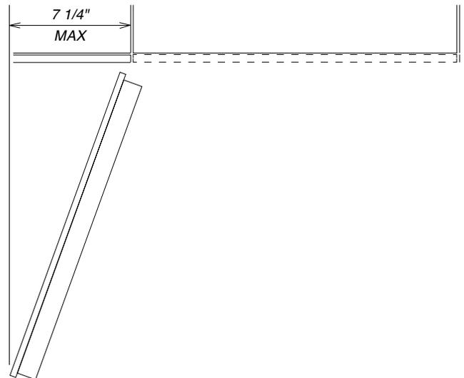
**NOTE:** Additional space needed depending on the thickness of front panels and handle used.
