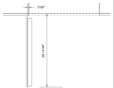
NOTE: Additional space needed depending on the thickness of front panels and handle used. Freezer units cannot be stop pinned at 90°
