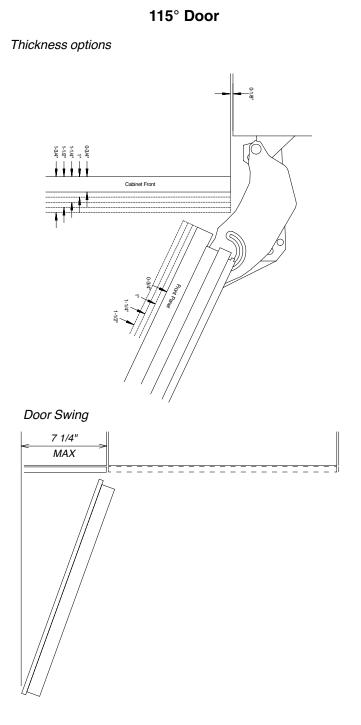
NOTE: Additional space needed depending on the thickness of front panels and handle used. Freezer units cannot be stop pinned at 90°
