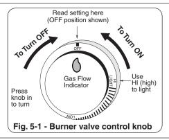
For your convenience and safety; when the control knob is in the ON position, the gas flow indicator will change from blue to red. (Red indicates gas flow.) See Fig. 5-1.
