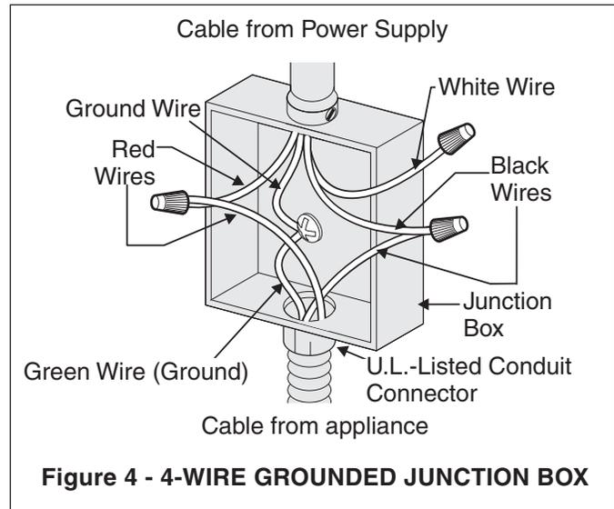
**⚠ WARNING** If connecting to a 4-wire power supply cable electrical system, the appliance frame connected ground wire **MUST NOT** be connected to the neutral wire of the 4-wire electrical system.
