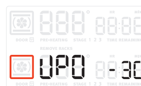
Figure 30: Oven temperature set 30^{\circ} lower than default
