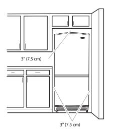
Allow at least 3 in. (7.5 cm) of air space at the top and on both sides of the freezer and 1 in. (2.5 cm) between the back of the freezer and the wall. If the freezer is to be against a wall, leave extra space on the hinge side so the door can open wider.
