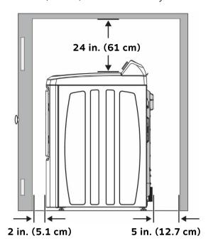
o If the dryer is installed in a closet, the door must have two unobstructed air openings with a combined total area of at last 72 in.² (465 cm²) and at least 3 in. (7.6 cm) of clearance at the top and bottom. A slatted door that meets these requirements is acceptable.
