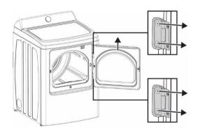
3. Remove the screws for the locker cover on the right side of the dryer and the screws for the locker on the left side of the dryer.
