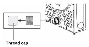
3. Apply a pipe joint compound or 1.5 in. (3.8 cm) wraps of thread seal tape over all threaded connections.
