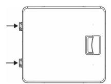
10. Align the hinges on the door with the hinge screw holes on the front of your dryer, then secure the door with the four screws you previously removed.
