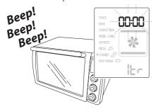
Turn the TOAST COLOUR/TIME dial (G) to adjust up to 10 additional minutes, if necessary, and press the START/STOP button (H) at the end of time, the control will turn off the oven.
