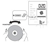
Turning TEMPERATURE/PIZZA SIZE/SLICES/TRAY dial (M) is possible to select "1tr" mode (1 tray of biscuits) or "2tr" mode (2 trays of biscuits).
