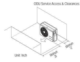
Figure 29: ODU Service Access Clearance - Multiple Units.
