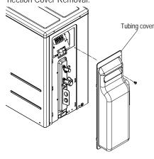
Figure 40: LSU240HEV1 Outdoor Unit Connection Cover Removal.
