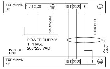
Figure 53: Terminal Block Wiring Diagram LS090HXV, LS120HXV LSU090HXV, LSU120HXV
