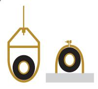
Figure 34: Typical Pipe Support Location—Change in Pipe Direction
