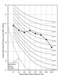
Figure 3: Sound Pressure Levels for Mega 115V Outdoor Units.
