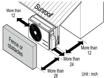
When placing the outdoor unit under an overhang, awning, sunroof or other "roof-like structure", observe the clearance requirements (as shown in Figure 27) for height in relation to the unit. This clearance ensures that heat radiation from the condenser is not restricted around the unit.
