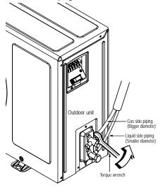
Figure 43: LSU180HEV1 Outdoor Unit Piping Connection.
