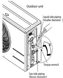
Figure 44: LSU240HEV1 Outdoor Unit Pipina Connection.
