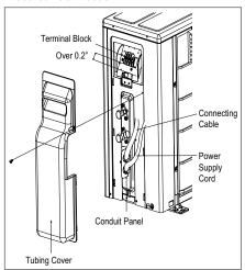
Figure 48: LSU240HEV1 Outdoor Unit Electrical Connection.
