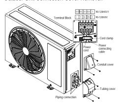
Figure 39: LSU180HEV1 Outdoor Unit Connection Cover Removal.
