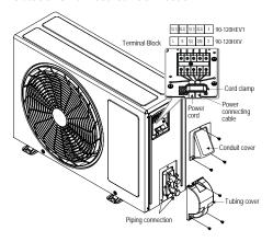
Figure 47: LSU180HEV1 Outdoor Unit Electrical Connection.
