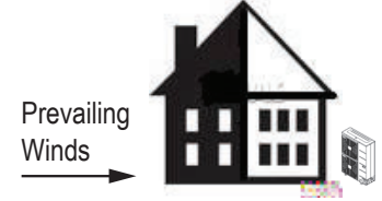
Figure 32: Leeward Side of the Building.
