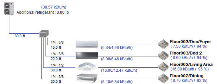
Figure 1: LATS Example (Tree Diagram; Illustrative Purposes Only. System will Vary Depending On Model).
