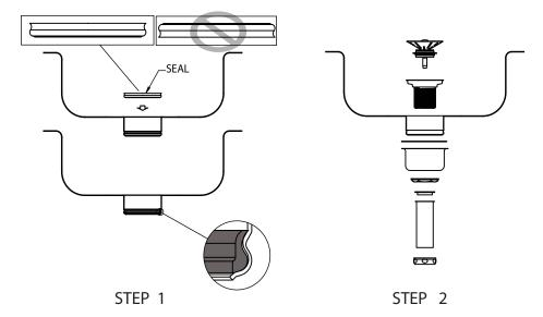
MAKE SURE THE SEAL IS CORRECTLY INSTALLED WITH THE PROPER ORIENTATION. INCORRECT INSTALLATION MAY ALLOW LEAKS AND VOID THE WARRANTY.
