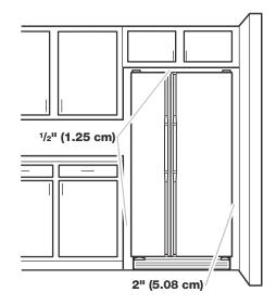
To ensure proper ventilation for your refrigerator, allow for 1/2" (1.25 cm) space on each side and at the top. When installing your refrigerator next to a fixed wall, leave 2" (5.08 cm) minimum on each side (depending on your model) to allow for the door to swing open. If your refrigerator has an ice maker, allow extra space at the back for the water line connections.
