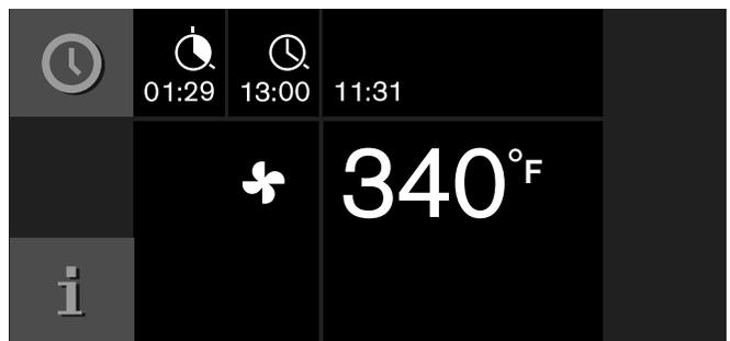
One minute before the end of cooking time, the remaining time will be magnified on the screen.
