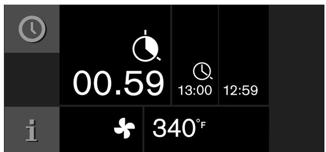
The appliance will turn off after the cooking time has ended. The ⌚ symbol will pulse and a signal will sound. It will stop when you touch the ✓ symbol, open the appliance door, or set the program selection to 0.
