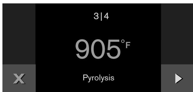
After 3 hours, a signal sounds. A message will appear on the screen. Once the appliance is cool, wipe out the remaining ash from the oven with a damp cloth.
