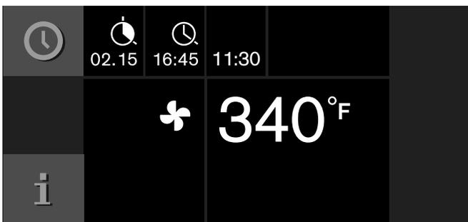
The appliance will go on standby. The screen will display the mode, temperature, cooking time, and end of cooking time. The appliance will start at the calculated time and will turn off automatically once the cooking time has run out.
