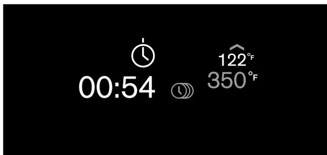
The program will begin with the pre-set warm temperature without light, then advance to the programmed temperature with light until the end of the set date and time, and then maintain the pre-set warm temperature for 60 minutes.
