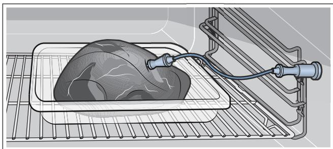
If there are several pieces of food, stick the core temperature probe into the middle of the thickest piece.
