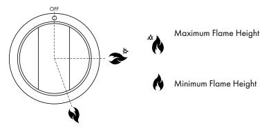
Maximum temperature setting/recommended control knob position for burner ignition.
