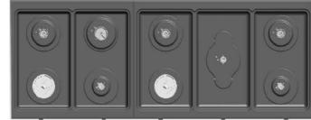
Dual Burner LPG: 1.27 - L20 NG: 2.38 - N21 Auxillary Burner LPG: 0.65 - L6 NG: 1.04 - N6 Dual Burner LPG: 1.27 - L20 NG: 2.38 - N21 Fish Burner LPG: 1.08 - L15 NG: 1.79 - N15
