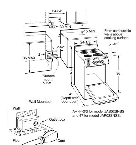
Recommended acceptable electrical outlet area. Orient the electrical receptacle so the length is parallel to the floor.
