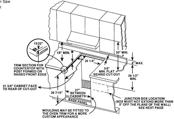
★ IF NEEDED, BUILD UP SIDES OF CUTOUT TO A MIN. OF 1 1/2" TOTAL THICKNESS (FULL DEPTH OF CUTOUT).
