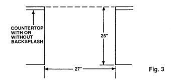
NOTE: If the distance from the back wall to the front of the counter backsplash (Dimension A in Fig. 4) is greater than 1 1/8", there will be a small gap between the wall and the edge of the backguard. This is normal and should not be visually objectionable (See Figs. 3 & 4).
