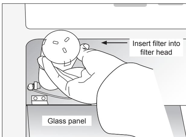
5. Remove the packaging on the new water filter cartridge and insert it into the filter head, located either to the right or left of the lighting system. Gently rotate the filter clockwise 1/4 turn, until it locks into place.
