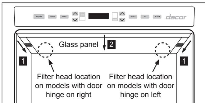
4. Remove the packaging on the supplied water filter cartridge and insert it into the filter head, located either to the right or left of the lighting system. Gently rotate the filter clockwise 1/4 turn, until it locks into place.
