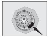
When this indicator light comes on, you must refill special salt. Only use special dishwasher salt in your machine to soften the water. The salt content can be read on the container for the salt. When the visual fill indicator is dark, there is enough salt in the container. When the color is light, open the container and add dishwasher salt.
