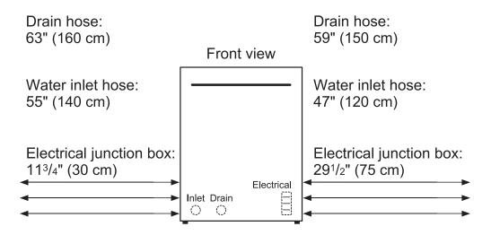
All connections are at the rear of the appliance. Extension for drain hose available as accessory. Power cord for connection to electrical outlet (3-prong plug) available as accessory.
