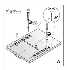
5. Attach the two mounting brackets to the wooden door with 4 screws (Ø  $^{1}$ /8" x  $^{5}$ /8" (Ø 3.5mm x 14mm) (Figure **A**).
