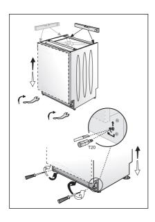
Adjust the front foot level with the adjusting wrench to balance and raise the dishwasher to the enclosure height.
