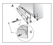
If the enclosure height is above 33<sup>1</sup>/<sub>16</sub>" (840mm) use "o" and "p" labelled toe kicks together. Make sure the slotted toe kick "p" is on the outside so you can adjust height of the toe kick. Installation should be done following the steps illustrated in the figures A, B and C respectively.
