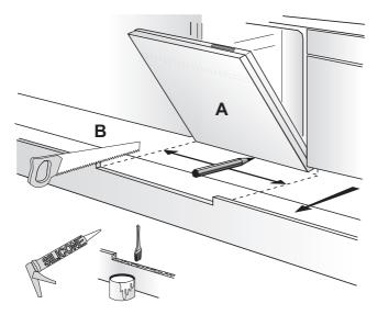
11. Check whether the bottom of the door hits the toe kick of the kitchen cabinet (**A**).
