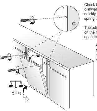
Check the door tension of the dishwasher: If the door closes too quickly or if the door falls open, the spring tension needs to be adjusted.
