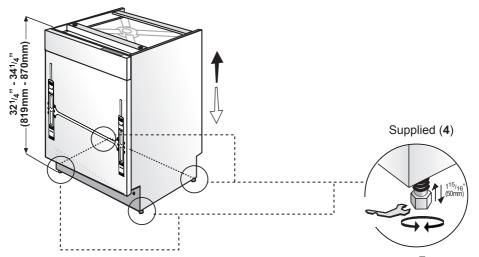
If the height of the enclosure is  $33^7/16$ " to  $34^1/4$ " (850mm - 870mm) use short supports as shown in the figure.
