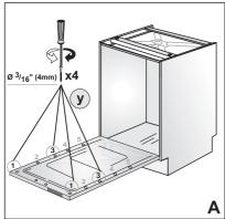
8. Using the four screws Ø  $^3/_{16}$ " x  $^{11}/_{16}$ " (Ø 4mm x 43mm) provided, attach the wooden door to the dishwasher at position 1 and 3 (Figure **A**).
