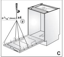
10. Tighten the screws in position 1 and 3 completely after the final alignment (Figure C).
