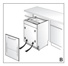
6. Mount the wooden door onto the dishwasher with the plastic mounting brackets which you have attached (Figure **B**).
