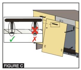
Before mounting the wooden door on the dishwasher, mount the handle on the wooden door as in figure C.
