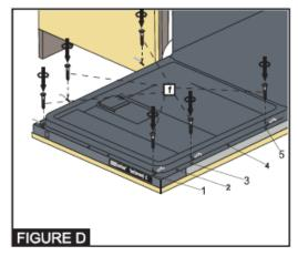
As shown in Figure D, the 5/32" x 53/32" (4mm x 42.5mm) screws are installed in positions 1,111 and V.
