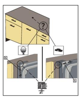
Mounting brackets previously fixed to the dishwasher are also fixed in the cabinetry with 5/32" x 19/32" (4mm x 15mm) screws.
