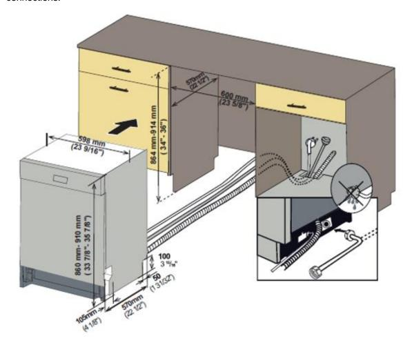
CAUTION: Make sure all hoses are pulled through the side openeing of the cabinet. No hoses should be kinked and ensure all slack is taken out, as shown above.
