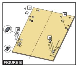
As shown in Figure B, the 5/32" x 27/32" (4mm x 21.5mm) screws are installed in positions III.
