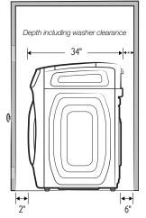
\*Required spacing (External exhaust elbow may require additional space.)
