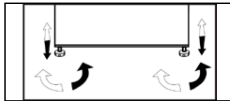
Legs that Stabilize on Uneven Surfaces
