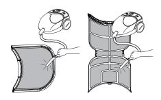
3 If the lint filter has become very dirty or clogged with fabric softener, wash the lint filter in warm, soapy water and allow it to dry thoroughly before reinstalling.
