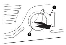
Press the tabs on the knockout 3 and carefully remove the knockout for the desired vent opening. (Right-side venting is not available on gas models.) Press the adapter duct **4** onto the blower housing and secure to the base of the dryer as shown.
