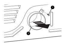
Press the tabs on the knockout and carefully remove the knockout for the desired vent opening. (Right-side venting is not available on gas models.) Press the adapter duct onto the blower housing and secure to the base of the dryer as shown.
