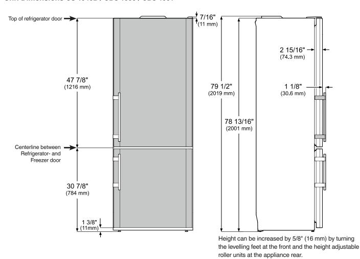
29 7/16" (747 mm) 23 7/16" (595 mm) 24 13/16" (630 mm) 52 5/16" (1328 mm) Allow door swing clearance at locations next to a wall. The refrigerator door must open 145° to a minimum of 90° to allow the crispers to open and the shelves to be removed. 90° It ist possible to limit the door
