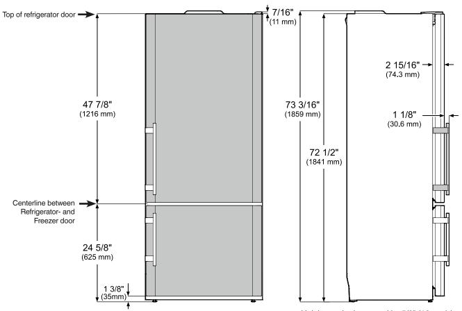
Height can be increased by 5/8" (16 mm) by turning the levelling feet at the front and the height adjustable roller units at the appliance rear.
