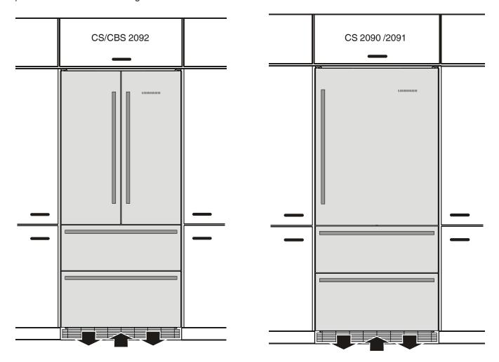
The cover grill provided with the appliance must be used for the ventilation opening. This grill must not be covered by toe kick or other trim.
