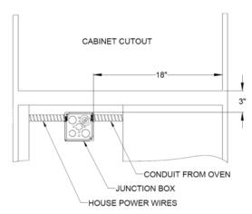
Move the oven with flexible conduit/wires close to the cabinet cutout and feed the wires and conduit through the rectangular cutout located at the rear end of the cabinet cutout base. 4. Feed the wires in to the junction box and connect the conduit to the junctions box using agency 1/2" conduit connector.
