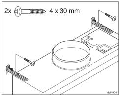
Drill respective holes and screw the fixing brackets to the wall or the
