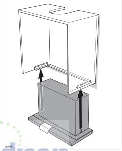
Insert the hood into the cabinet from below and until the spring clips click into place.
