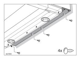
Connect the space bar from the rear with 4 plastic rivets at the hood rear side.
