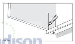
■ At the front edge of the spacer strip mined breaking point of the next and draw a vertical line on left and right side of the inside cabinet.
