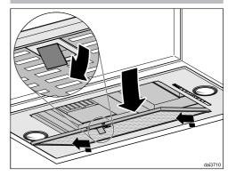
■ To take out a grease filter, release the locking clip on the filter, lower the filter approx. 45°, unhook it at the back and remove it.
