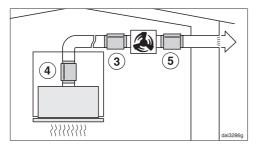
To minimise noise from the motor in the kitchen, the silencer should be positioned in front of the external motor ③ if possible, or, if the ducting is long, above the exhaust connection inside the rangehood ④. In the case of an external motor located inside the house, fitting a silencer behind the external motor ⑤ reduces the noise of the motor outside the house.
