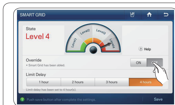
[Turn Off Override, Turn On Smart Grid]
