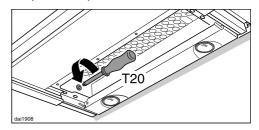
■ Note for dismantling the hood: Removing the screws on the left and right inside the cabinetry releases the spring mounts, allowing the appliance to be removed from the unit.
