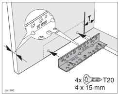
■ The brackets are designed for <sup>5</sup>/<sub>8</sub>" and <sup>3</sup>/<sub>4</sub>" (16 and 19 mm) thick unit sides. Orientate the bracket so that the vertical depth matches the thickness of the unit side. Screw the brackets onto the right and left inside walls of the housing unit as shown. The back edge of the bracket should align with the vertical line drawn up from the front of the spacer strip and the lower edge should align with the lower edge of the cabinetry side wall.
