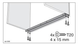
■ Secure the spacer strip underneath the sides of the cabinetry, flush with the rear wall.
