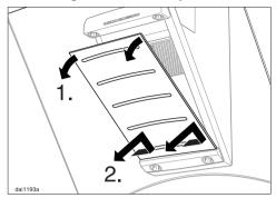
■ To remove the air intake panel gently pull out and downward, shifting the lower part a bit to the right. Lift it out of the latches.
