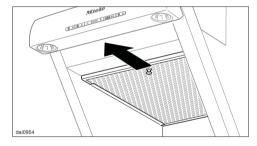
■ To remove the grease filter, pull on the lever. Support the grease filter so that it does not fall onto the cooktop.
