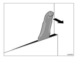
■ After removing the screws from the chimney, slide the lever between the chimney and the chimney extension and gently apply pressure to ease the chimney from its hooks.
