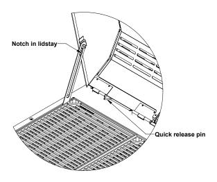
With the quick release pin removed, grasp the lid, pushing back on the center to clear the middle hinge and slide the lid away from the center of the grill until the outer hinge is free of it's pivot pin. Once the lid(s) have been removed they can be washed in warm, soapy water. Installation is reverse of removal.
