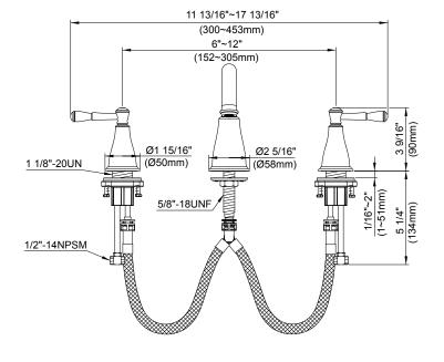
\* Installation method shown is for deck thickness of less than 1". If the installation is for deck thickness between 1" and 2", the sleeve nut needs to be reversed.
