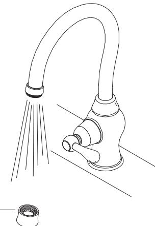
5. After installing faucet, remove aerator (1) and turn on water to remove any left over debris. Re-assemble aerator.
