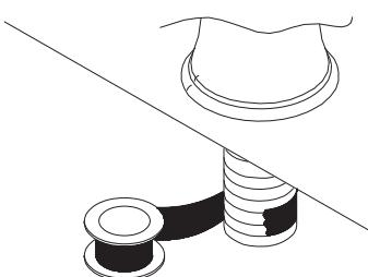
3. Apply pipe tape to threads.
