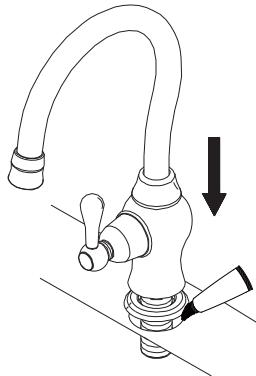
1. Apply silicone sealant around bottom of spout trim ring. Install faucet body and flange through top of sink.
