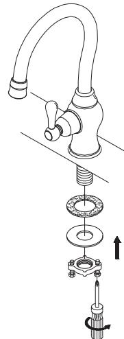
2. From underneath the sink, install the washers and lock nut. Tighten the screws on the lock nut to secure the body.
