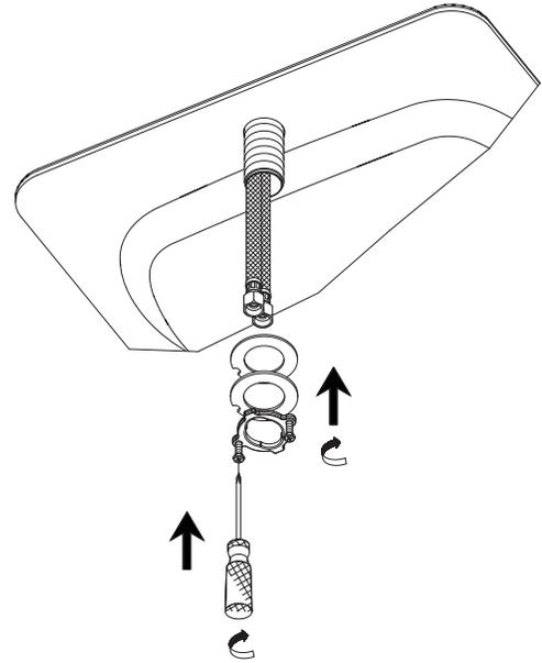
2. From underneath the sink, install washers and lock nut. Tighten the screws on the lock nut to secure the body.
