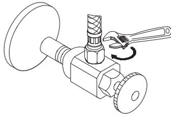
4. Tighten the hose onto water supply.
