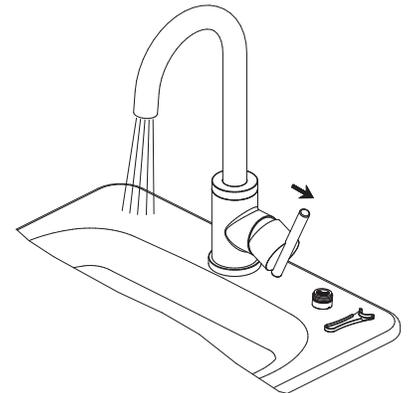
5. After installing faucet, turn on water to remove any left over debris.
