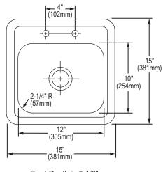
Bowl Depth is 5-1/8" Model D115152 Illustrated HOLE DRILLING CONFIGURATIONS
