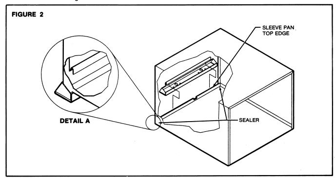
STEP 4. Push the trough down so that the sleeve pan edge seats in the trough lip as shown in Detail A.
