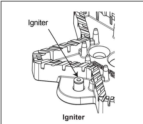
Each burner has its own electronic igniter that sparks when the burner is turned on. Each burner should light in 4 seconds or less. If a burner does not light, check to see that the burner cap is positioned correctly on the burner base.
