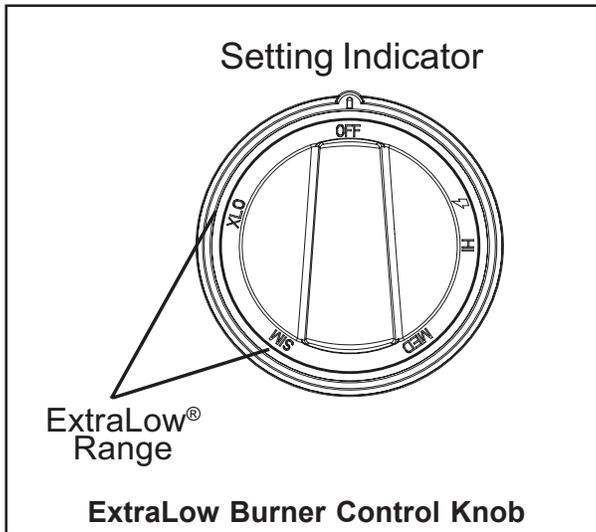
The drawing shows that the control knob has an additional range between the **SIM** and **XLO** settings. When the knob is set within this range, the flame cycles off and on. By varying the length of time the flame is off and on, the heat is reduced even further to cook delicate foods. For example, these very low settings are suitable for simmering and poaching, melting chocolate and butter, holding cooked foods at temperatures without scorching or burning, etc.
