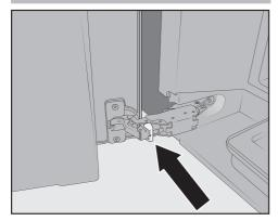
■ Remove the door opening limiters from the hinges, e.g., by prizing them out with a screwdriver.
