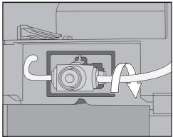
**Tip:** If necessary, screw the milk pipework backward at the connecting piece on the right-hand side.
