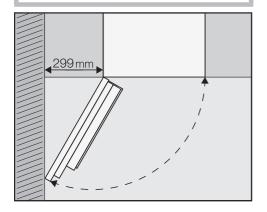
Check that there is a gap of at least 11 3/4" (299 mm) between the wall (or similar) and the coffee machine so that you can open the door wide enough to remove the left-hand bean container (minimum door opening angle of 120°).
