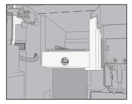
Remove the milk-valve cover: press on the recessed grip to unlock the cover. On the top right-hand side of the cover, you will find a pin for swiveling the cover out.
