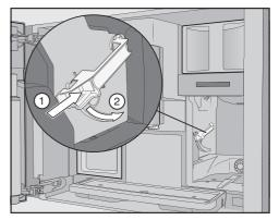
■ Press the button under the handle of the brew unit ① and, while doing so, turn the handle backward ②.
