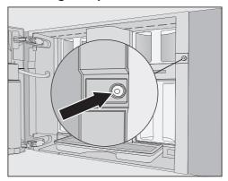
1 screw hole is fitted with a red silicone plug to protect the appliance against transport damage and secure the door during transport.
