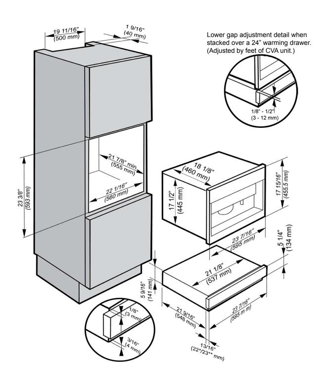
PLEASE NOTE: The vent cut out must only be at the top of the niche to prevent condensation inside the door and inner components that the customer can see when opening the door.
