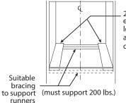
2 x 4 or equivalent runners level with bottom of cutout and flush with sides of cutout or solid bottom floor.
